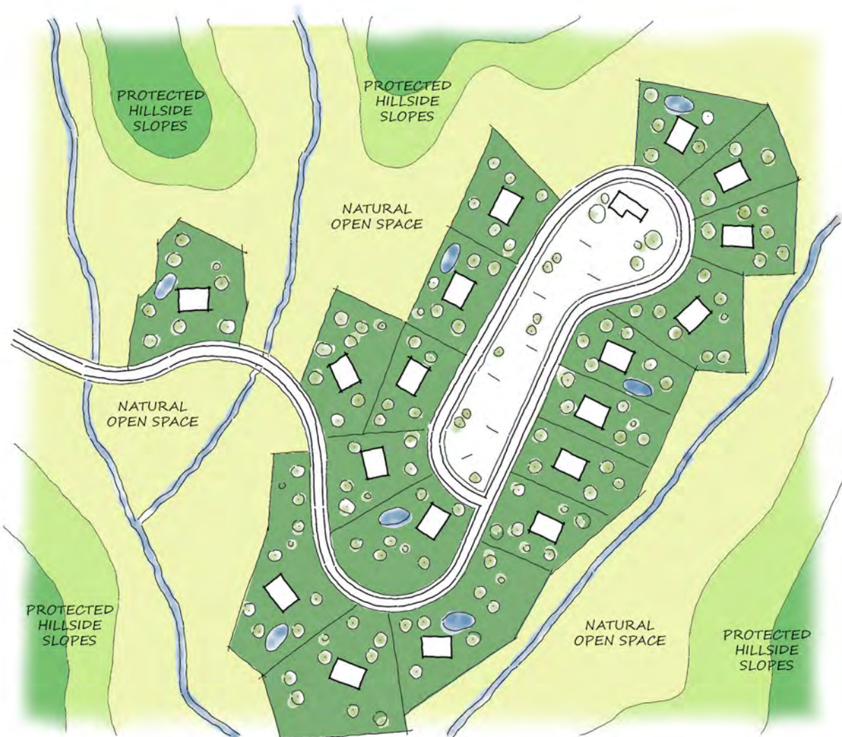
Figure 45. Diagram illustrating the preference for clustering of development, retention of natural areas, and protection of hillside slopes [See 4.9.5.5, 6 & 9]
