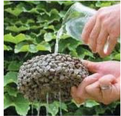
Figure 5. Pervious concrete allows water to flow through. Photo courtesy of the National Ready Mix Concrete Association.
