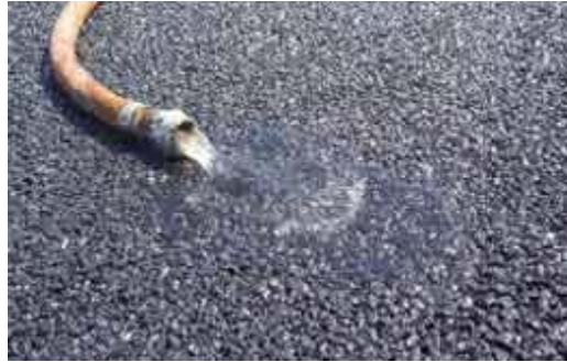
Figure 12. Porous asphalt allows water to flow through it. Photo courtesy of the National Asphalt Paving Association.
